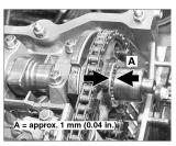
Engine and cylinder head service, including Double VANOS timing chain setup and adjustment.
