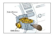
Learn about fascinating technologies inside the world's most successful hybrid vehicle, such as shift-by-wire system gear selector.
